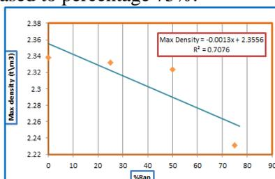
**Fig. 7.** Effect of Increasing RAP% on Unit weight.
