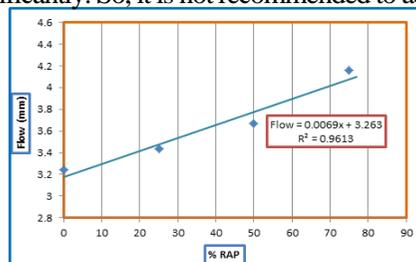
Fig. 9. Effect of Increasing RAP% on Flow.
