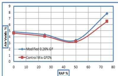
Fig. 14. Relationship between Air Voids and RAP % at 0.26% (GF)
