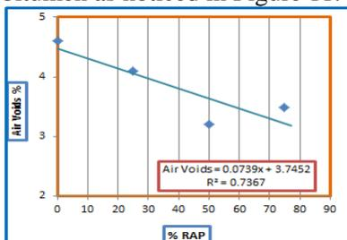
Fig. 10. Effect of Increasing RAP% on Air Voids
