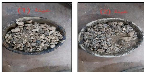
**Fig. 2.** Appearance of Coarse Aggregate from RAP
