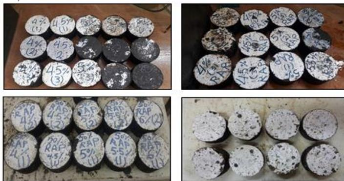
**Fig. 4.** Marshal Specimens for different bitumen percentage
