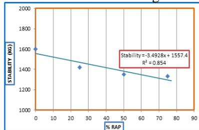
Fig. 8. Effect of Increasing RAP% on Marshall Stability
