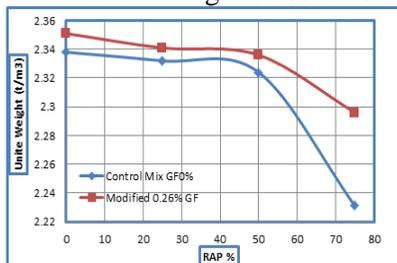
Fig. 12. Relationship between unite weight and RAP % at 0.26% (GF)
