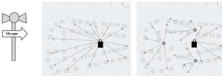
**Fig. 1.** (Left) Loudspeaker post, (Middle) Single Post distribution, (Right) Multiple Post Distribution (Source: Author)
