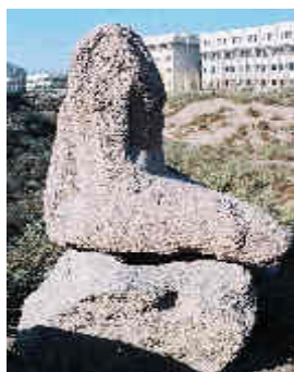
Fig. 4: The weathering and kaolinization of granite statues .
