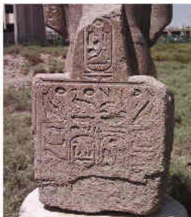
Fig. 9C: Shows scaling and exfoliation of granite statues.
