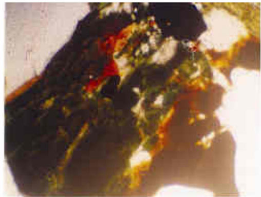
Fig. 12: Shows the alteration of biotite and plagioclase to iron oxyhydroxides (red colour) and chlorite (green colour).
