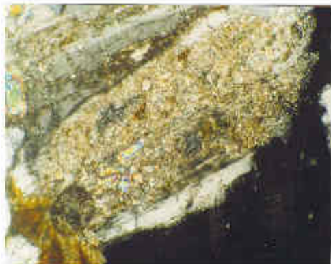
Fig. 13: Plagioclase is largely replaced by fine particles of sericite .
