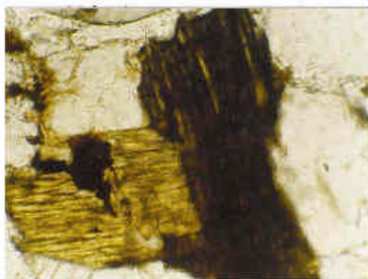
Fig. 15: The deformation of quartz and biotite. The cracks are filled by secondary material.
