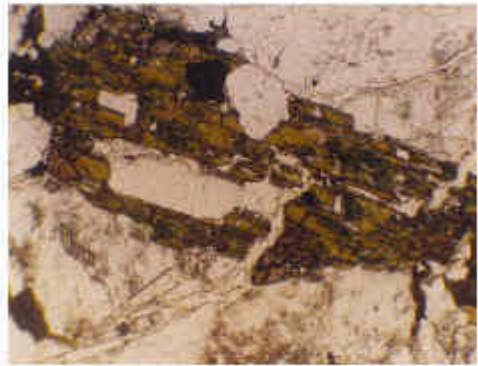
Fig. 17: The deformation and alteration of biotite to chlorite in particular through
