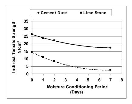
Figure 7: Effect of Moisture Conditioning Period on Indirect Tensile Strength.
