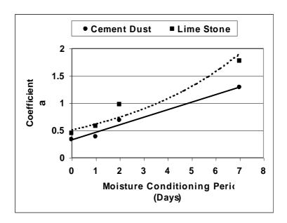
**Figure 4**: Variation of Compliance Coefficient (a) with the Change in Moisture Conditioning Period.
