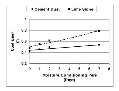
**Figure 5**: Variation of Compliance Coefficient (m) with the Change in Moisture Conditioning Period.
