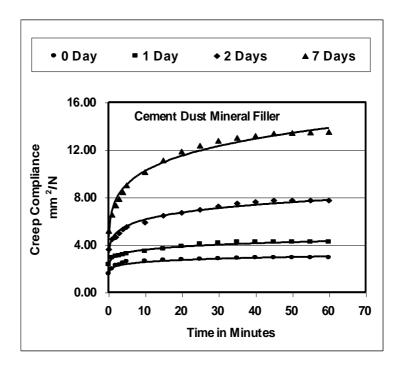
**Figure 3**: Creep Compliance Vs. Time at Different Conditioning Periods for Asphalt Mixture Containing Cement Dust Mineral Filler.
