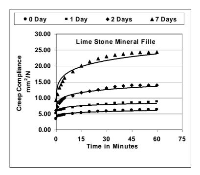
**Figure 2**: Creep Compliance Vs. Time at Different Conditioning Periods for Asphalt Mixture Containing Lime Stone Mineral Filler.
