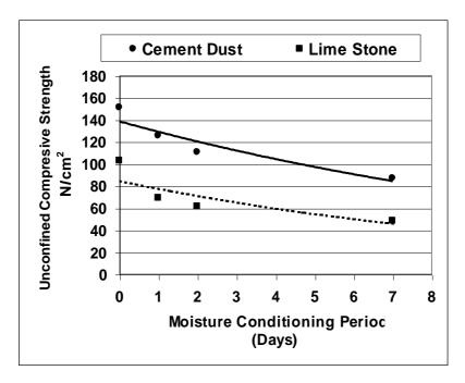
Figure 8: Effect of Moisture Conditioning Period on Compressive Strength.
