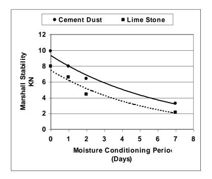
Figure 6: Effect of Moisture Conditioning Period on Marshal Stability.
