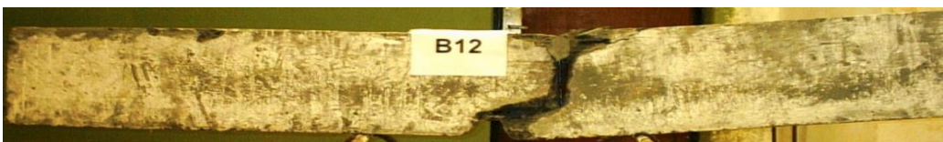
Fig. 2.f: Pattern of crack of the tested beam (B12).
