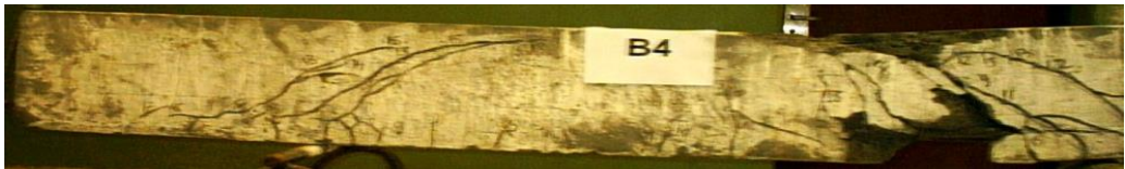
Fig. 2.d: Pattern of crack of the tested beam (B4).
