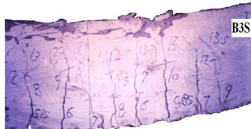
Fig. 6f: Failure shape of beam (B3S).
