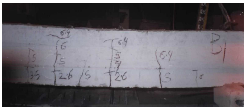
Fig. 5a: Failure shape of beam (B1).
