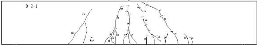
Fig. 6. Typical pattern of cracks for beam (B2-1) having f_{cu}=766 \text{ kg/cm}^2 and a/d=3
