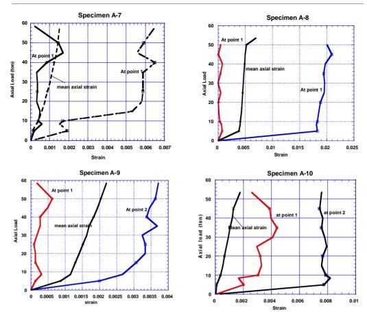
Fig. 5: Relations of axial load of the column and strain for specimens A-1 to A-12.
