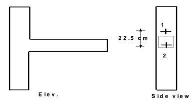
Fig. 4: Positions of the Measured Strain.
