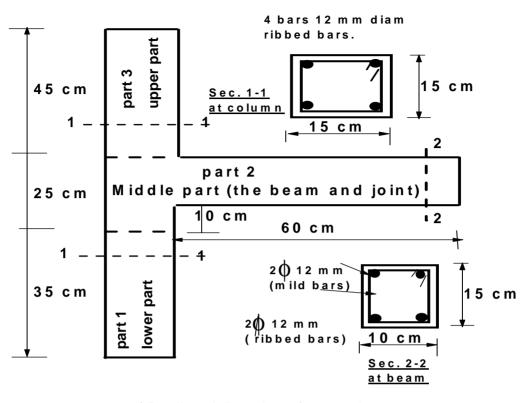
a) Details and dimensions of test specimens
