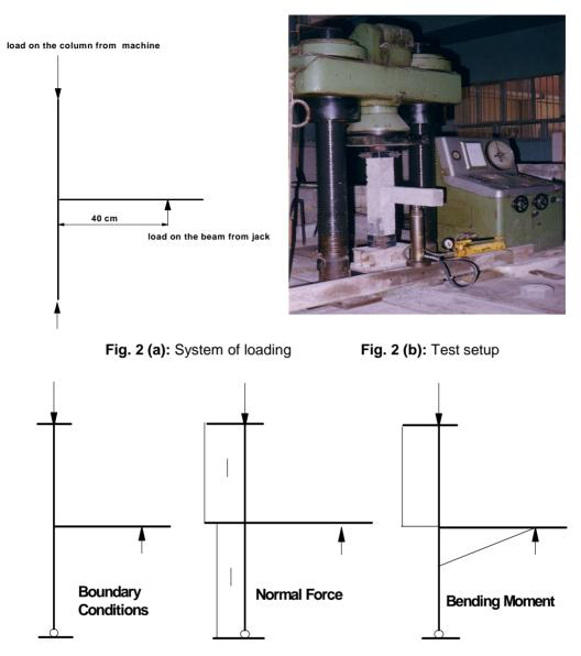
Fig. 3: Boundary conditions and straining actions of test specimen.
