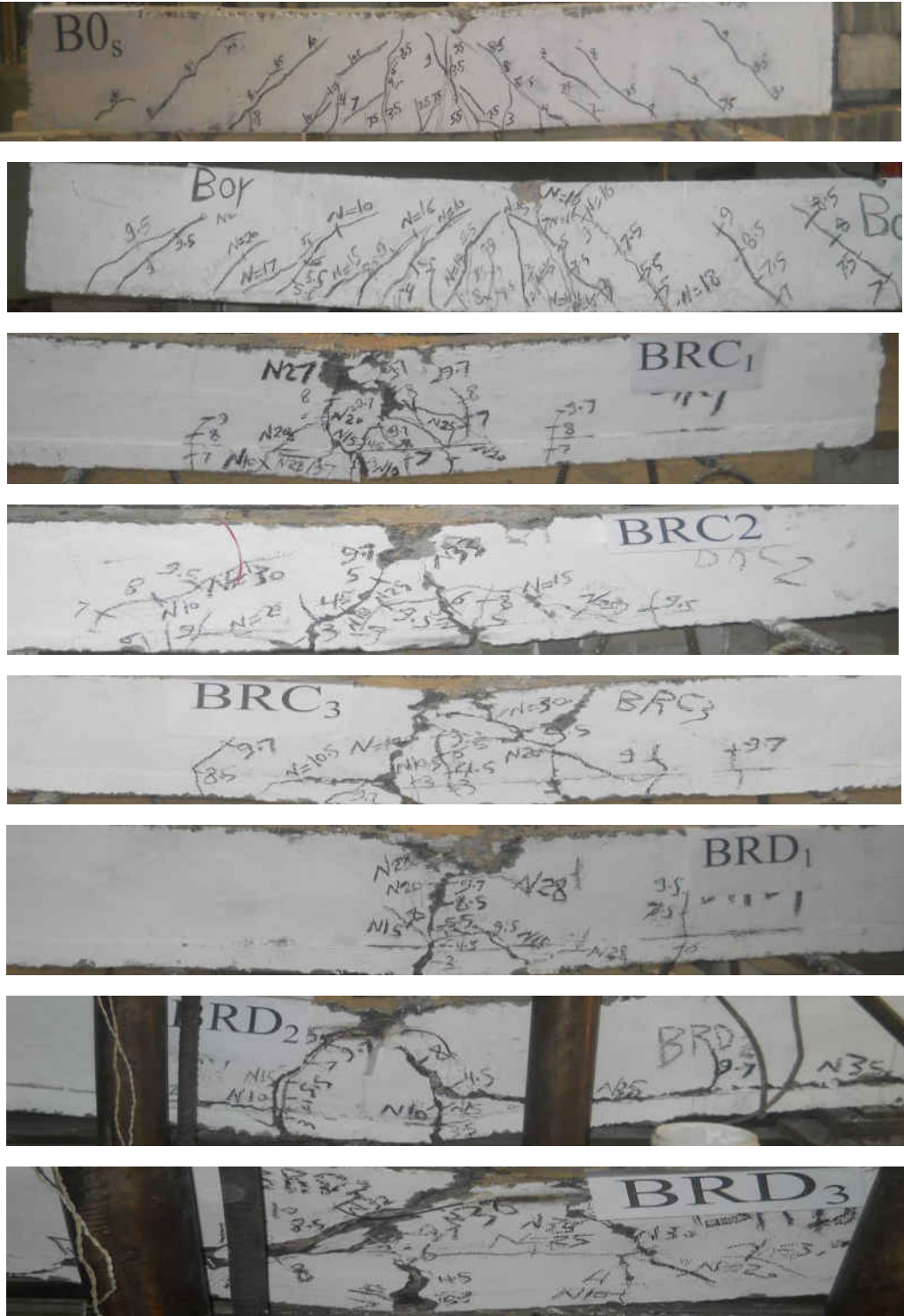
Fig. 5: Crack pattern and mode of failure of the tested beams
