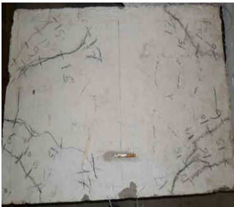
Fig. 6-B: Failure mode and cracks pattern for B2
