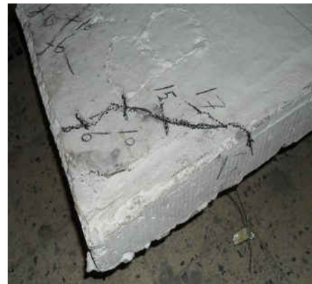
Fig. 6-B: Failure mode and cracks pattern for B2
