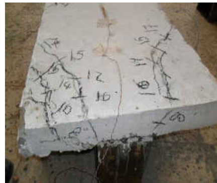
Fig. 6-A: Failure mode and cracks pattern for B1
