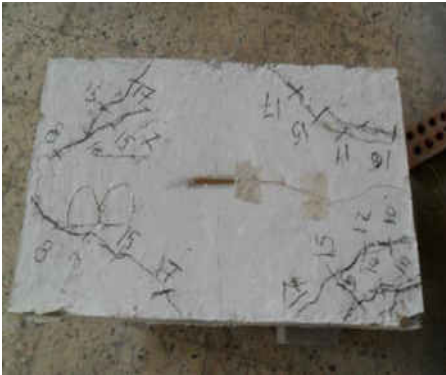
Fig. 6-A: Failure mode and cracks pattern for B1
