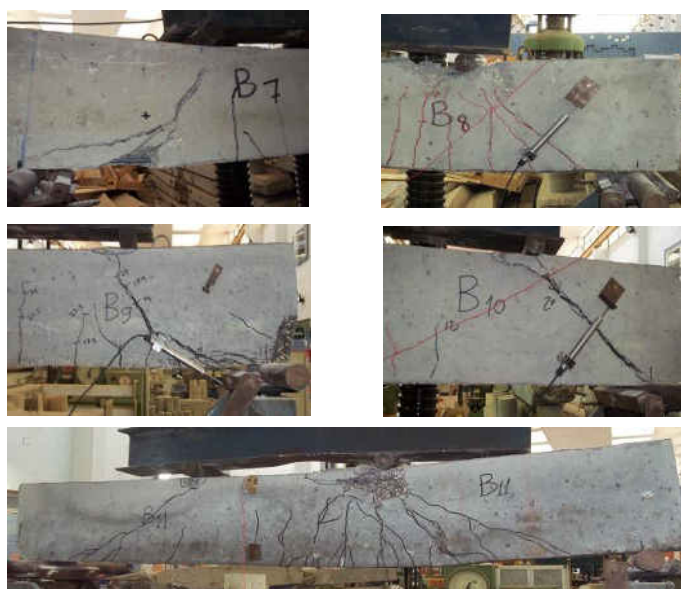
Figure (6): Failure Shapes of Beams of Group B
