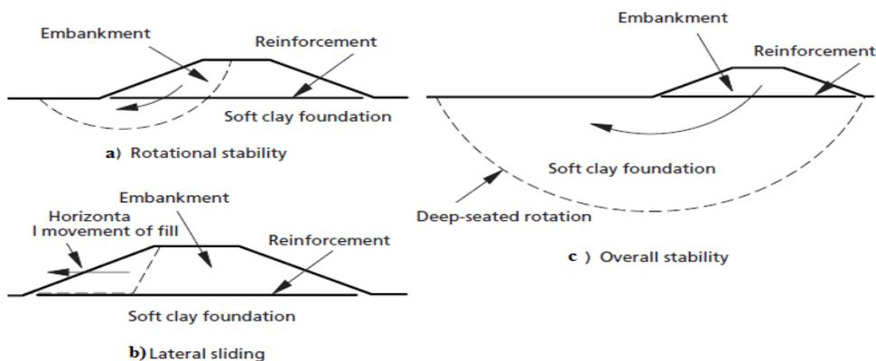
**Fig. 4:** The main failure modes for the reinforced embankment on soft clay (after BS 8006-1,2010)
