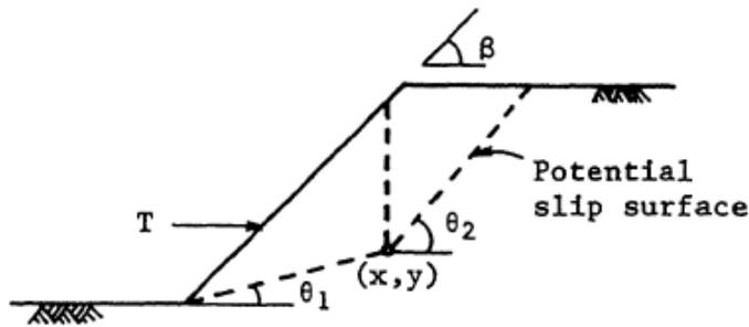
Fig. 5: The two-part wedge mechanism (After Jewell et al,1991)
