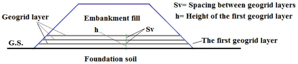
Fig. 10: Position of geogrid layers
