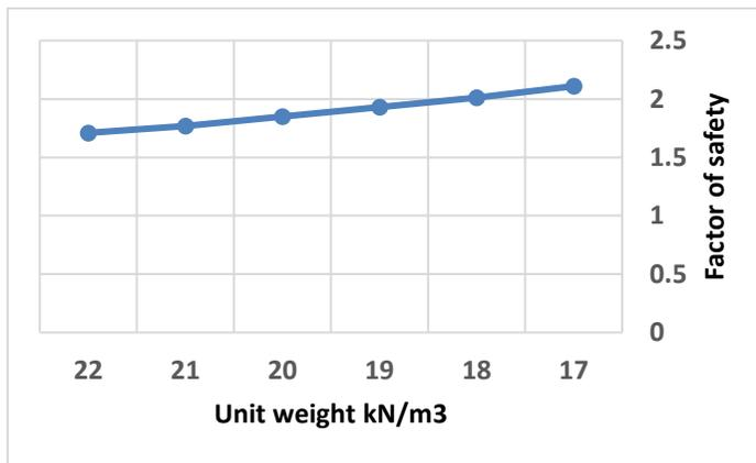
Fig. 16: The relation between the unit weight and the factor of safety for slope stability
