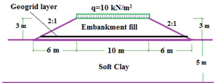
Fig. 7: Geometry of Model
