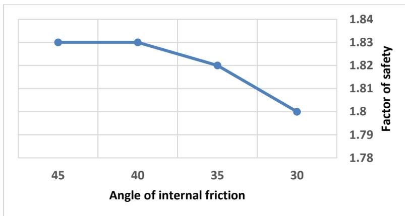
**Fig. 13:** The relation between the angle of internal friction and the factor of safety against lateral sliding
