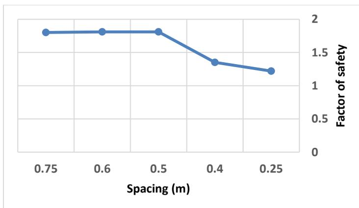
**Fig. 8:** The relation between geogrid spacing and the factor of safety against lateral sliding
