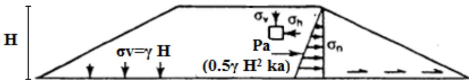
Fig. 17: Effect of the unit weight on embankment stability
