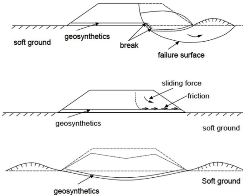
**Fig. 1:** Effect of Geosynthetics on the stability of embankment on soft soil (after the International Geosynthetics Society).
