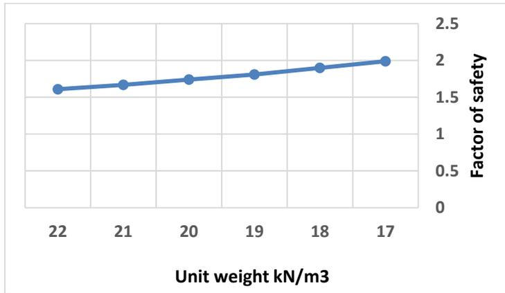
Fig. 15: The relation between the unit weight and the factor of safety against lateral sliding
