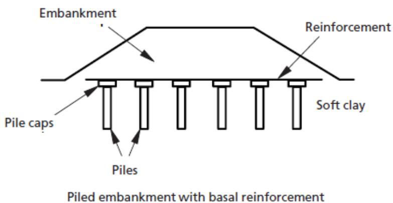
**Fig. 3:** Control both stability and settlement of embankment using reinforcement (after BS 8006-1,2010)
