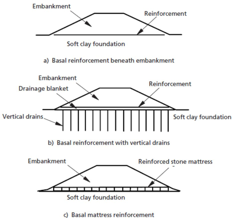
**Fig. 2:** Control only stability of embankment using reinforcement (after BS 8006-1,2010)
