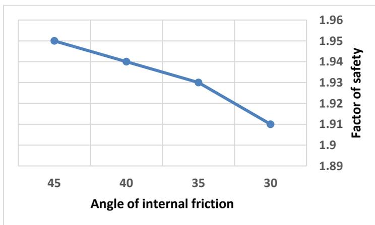
**Fig. 14:** The relation between the angle of internal friction and the factor of safety for slope stability
