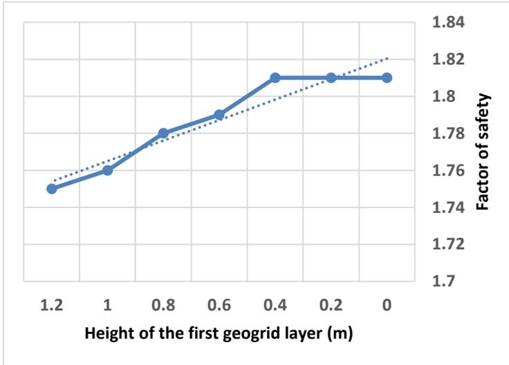
Fig. 11: Effect of the height of the first geogrid layer on the factor of safety against lateral sliding
