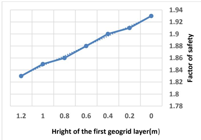
Fig. 12: Effect of the height of the first geogrid layer on and the factor of safety for slope stability
