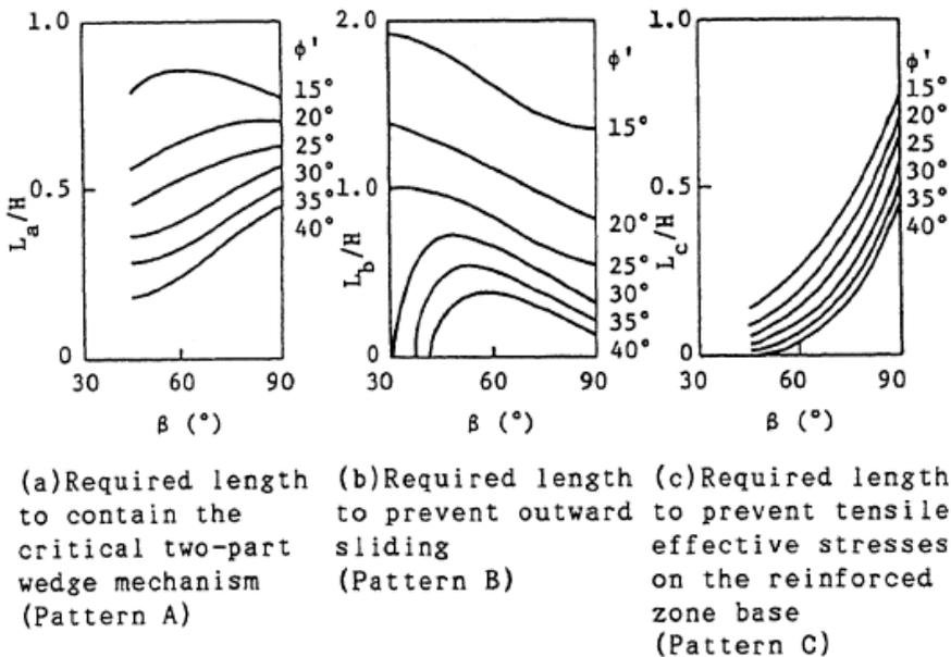
Fig. 6: Determination the reinforcement length (After Jewell et al,1991).
