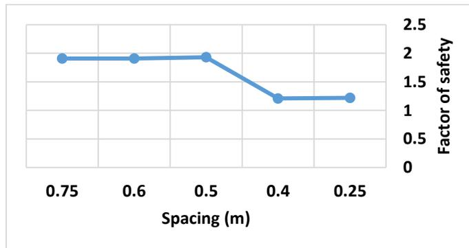
**Fig. 9:** The relation between geogrid spacing and the factor of safety for slope stability
