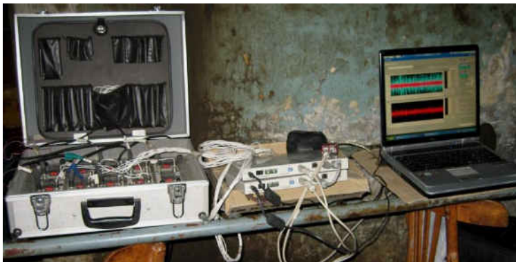
Fig. 3 Data acquisition system used to collect the dynamic test data
