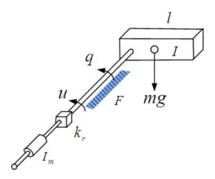
Fig. 4. One-link robot.
