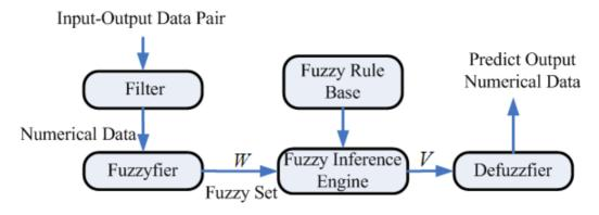
Fig. 1. Fuzzy input-output model.
