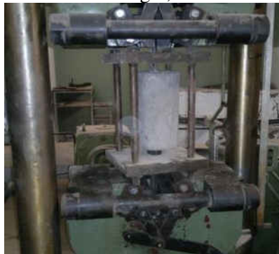
Fig. 4. Pull out bond strength test.
