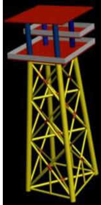
Fig. 3 Sketch map of the platform model
