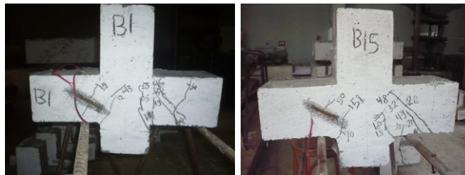
without horizontal stirrups 2Φ6 horizontal stirrups (e) Effect of horizontal stirrups
