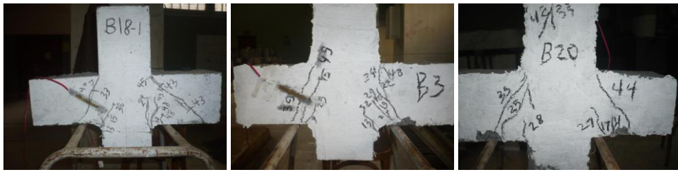
2Φ12 main reinforcement 2Φ16 main reinforcement 2Φ18 main reinforcement (c) Effect of main reinforcement
