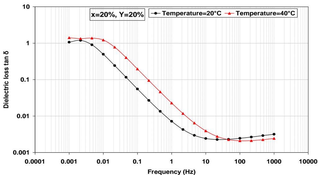
Fig. 10: Influence of transformer insulation temperature on frequency domain measurements of dielectric loss  $\tan \delta(\omega)$ .
