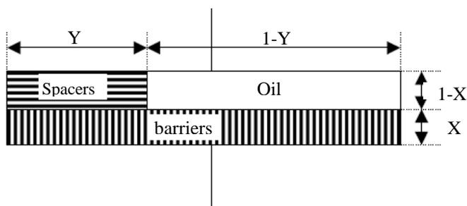
Fig. 3: Simplified insulation structure of a core type power transformer [10]
