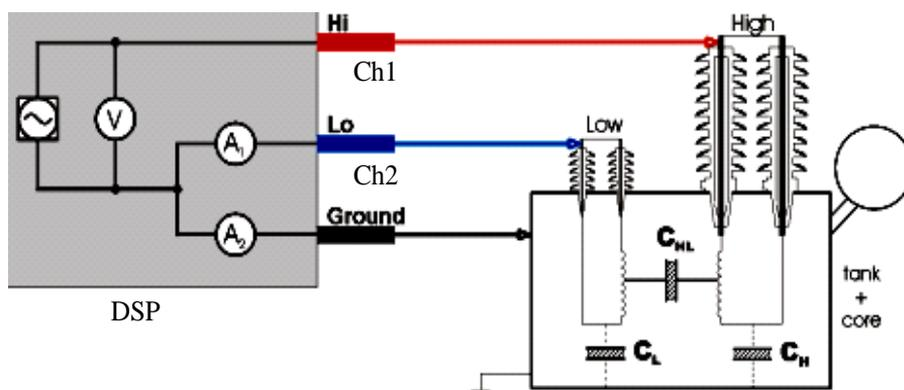
Fig. 4: Simplified diagram of capacitance measurement (frequency domain) for power transformer
