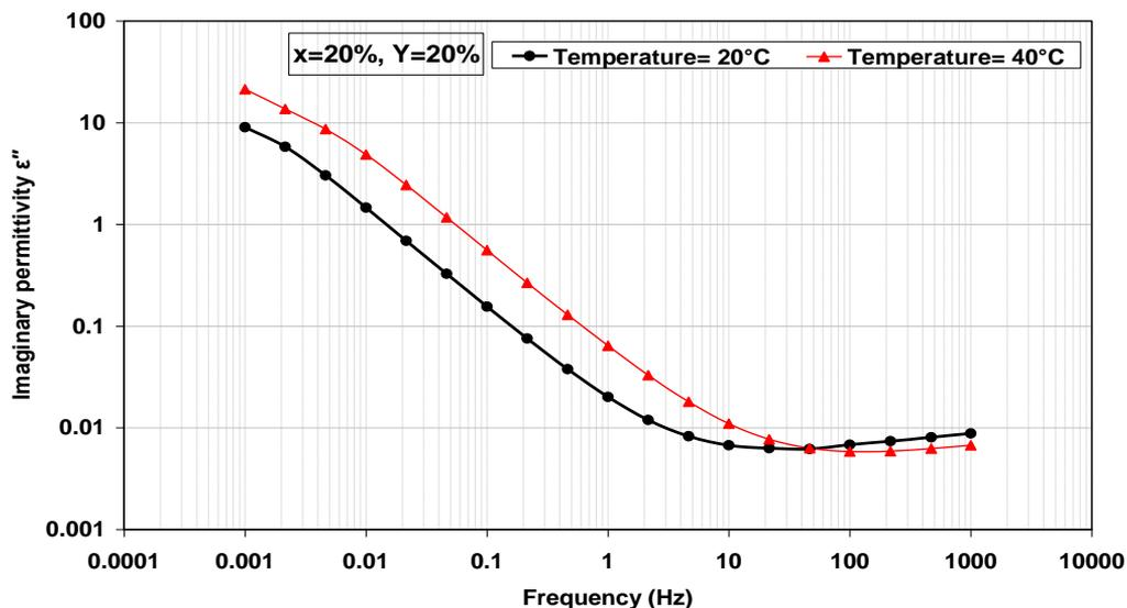
Fig. 9: Influence of transformer insulation temperature on frequency domain measurements of imaginary permittivity  $\epsilon''(\omega)$ .
