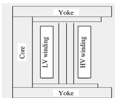
Fig. 1: Typical winding configuration of a power transformer
