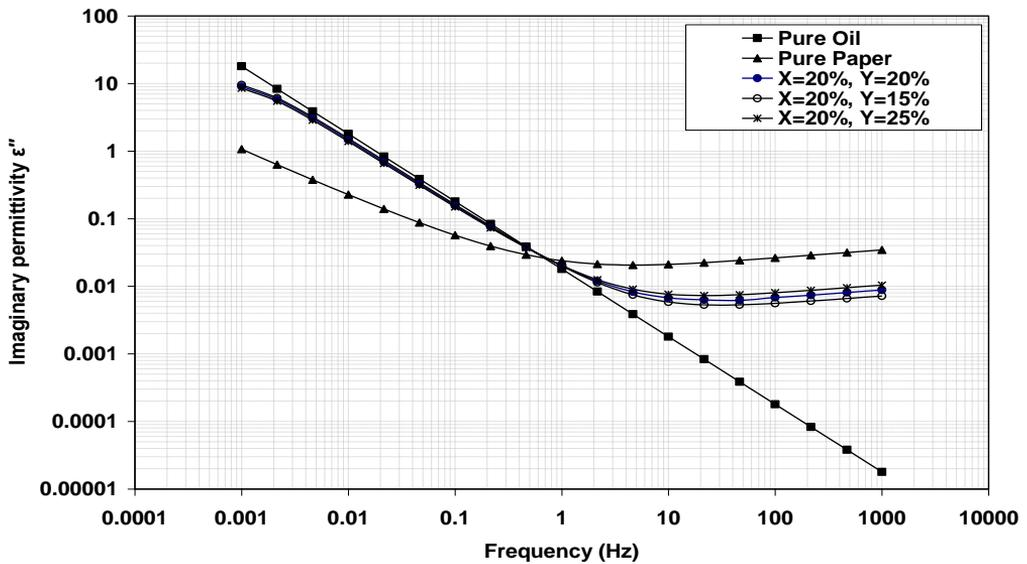
Fig. 6: Influence of transformer insulation geometry arrangement on frequency domain measurements of imaginary permittivity  $\epsilon''(\omega)$ .
