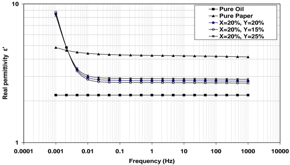
Fig. 5: Influence of transformer insulation geometry arrangement on frequency domain measurements of real permittivity  $\epsilon'(\omega)$ .
