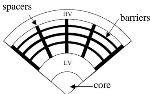
Fig. 2: Cross section of the main insulation of a core type transformer
