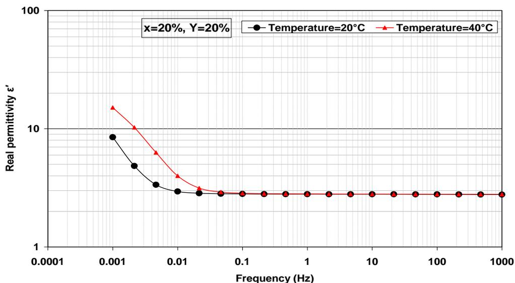
Fig. 8: Influence of transformer insulation temperature on frequency domain measurements of real permittivity  $\epsilon'(\omega)$ .
