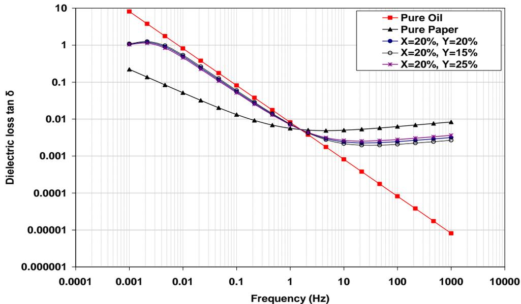
Fig. 7: Influence of transformer insulation geometry arrangement on frequency domain measurements of dielectric loss  $\tan \delta(\omega)$ .
