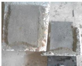
Fig(3-3): Effect of Curing pressures (CFRP sheet marked deeply in bonding agent)
