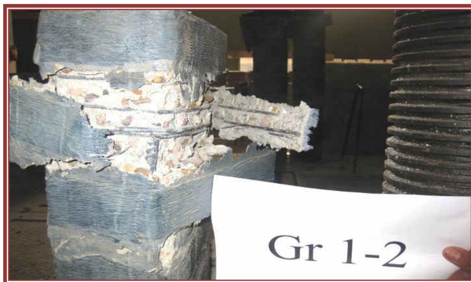
Failure mode, R.C. columns confined one and two layers ) ( FM 2)
