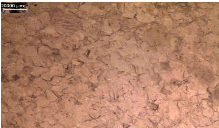
Fig. 3. Photo micrograph in White marble showing the Calcite
