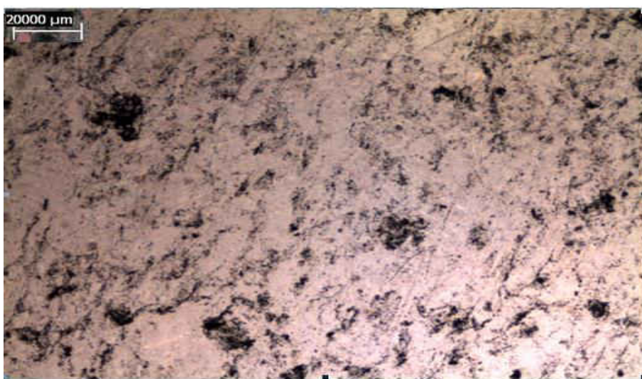
Fig. 1. Photo micrograph in Black marble showing the calcite
