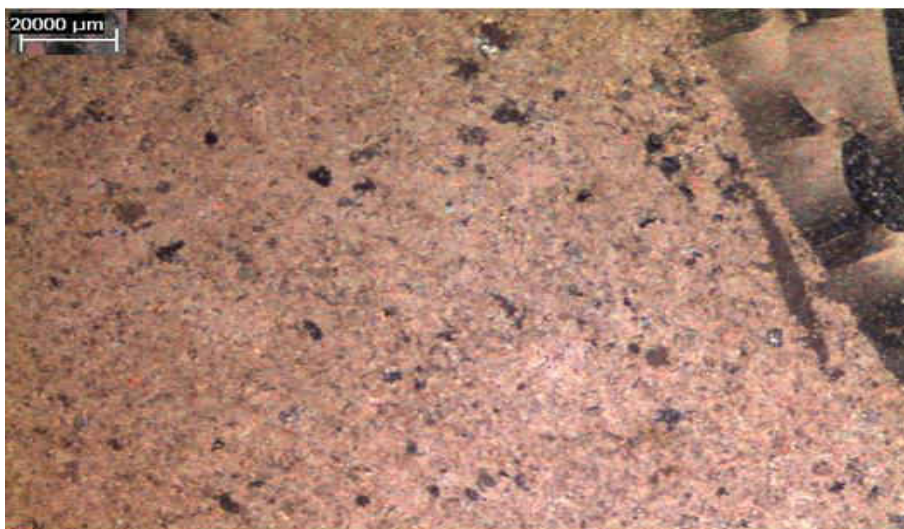
Fig. 8. Photo micrograph in Yellow marble showing the quartz.
