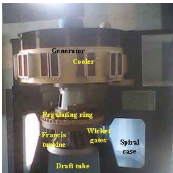
Fig. 2. Sectional model of the hydro-power unit.
