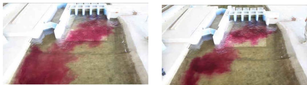
Fig. 11. Observed lateral currents downstream the navigable lock
