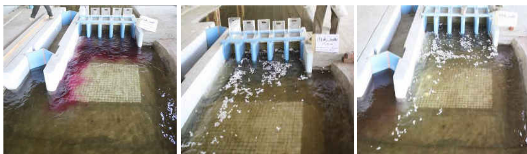
Fig. 10. Observed flow and the hydraulic jump over the proposed sill structure
