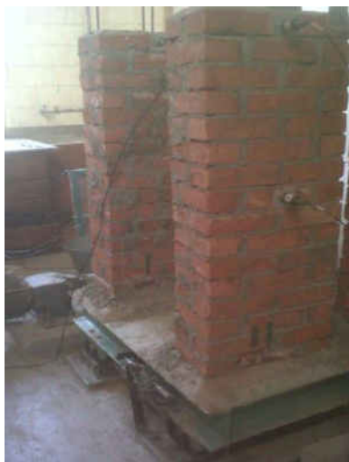
Fig. 2. Masonry piers built on shaking table.
