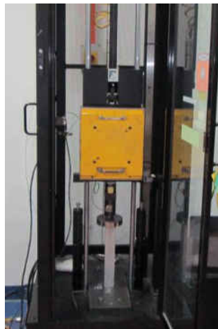
Fig. 5. Specimen positioning and loading arrangement for dynamic loading
