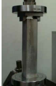
Fig. 4. Specimen positioning and loading arrangement for static loading
