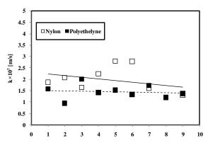
Fig. 10.Overall membrane mass transfer coefficient.
