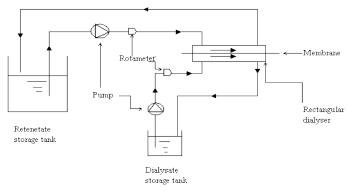
**Fig. 1.** Schematic and flow diagram of the test rig.
