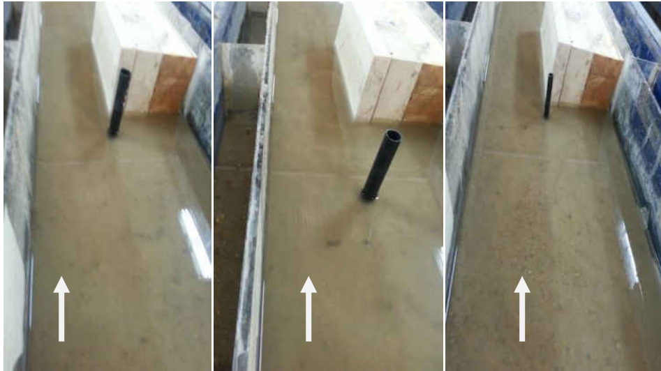
Photo 1. Different diameters and positions of pile
