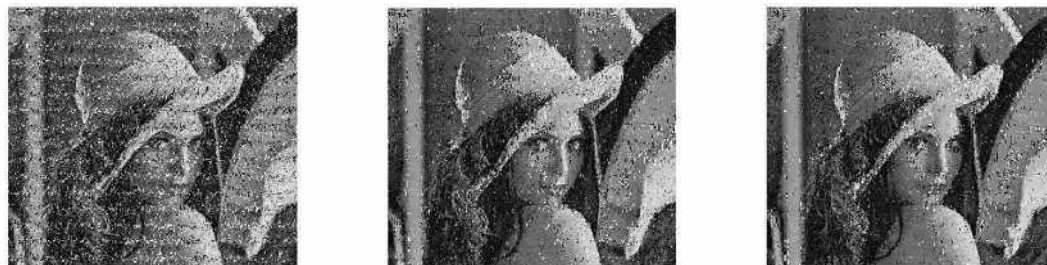
Fig. 26. CP-OFDM, and ZI-OFDM with denoising when 25% fading delay and SNR=0db Gaussian noise (a) received image without denoising PSNR=14.8022 (b) received image with the CP-OFDM denoising PSNR=17.7931 (c) received image with the proposed system PSNR=18.2096
