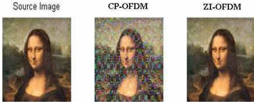
Fig. 14. Mona Lisa Image as a source and received images from CP-OFDM and ZI-OFDM systems at path gain= -0.26 dB and delay = 10^{-5}
