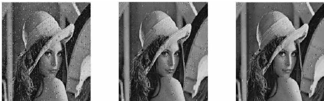
Fig. 25. CP-OFDM, and the proposed system when 1% fading delay and SNR=5db Gaussian noise is added (a) received image without denoising PSNR=21.7663 (b) received image with the CP-OFDM denoising PSNR=24.3318 (c) received image with the proposed system PSNR=25.4752
