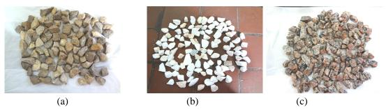
**Fig. 2.** Crushed aggregated used in this study, a: phosphate wastes, b: marble, c: granite.
