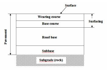
Fig. 1. Structural layers in road construction [12, 13, 17].
