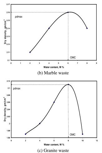
**Fig. 3.** The relation between dry density and water content for the three studied waste materials: phosphate, marble, and granite.
