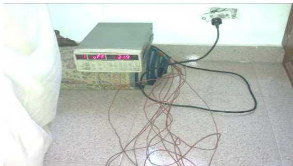
(c) The 12 thermocouples connected between the scanning thermometer instrument sockets and measuring points
