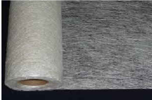
Fig. 1. glass fiber used in strengthening of beams.
