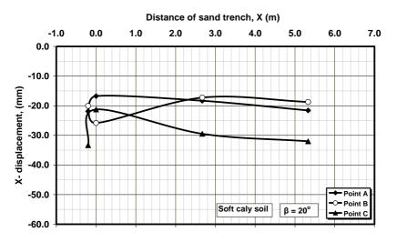
**Figure 7.** Horizontal displacements for slope ( $\beta = 20^{\circ}$ ) due to strip footing, case of soft clay (C = 10 KN/m<sup>2</sup>)
