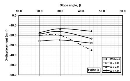
**Figure 8.** Horizontal displacements versus slope angle  $\beta$  for point B due to strip footing, case of soft clay (C = 10 KN/m<sup>2</sup>)
