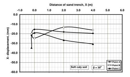
Figure 6. Horizontal displacements for slope ( $\beta = 30^{\circ}$ ) due to strip footing, case of soft clay (C = 10 KN/m<sup>2</sup>)
