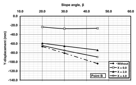
Figure 12. Vertical displacements versus slope angle  $\beta$  for point B due to strip footing, case of soft clay (C = 10 KN/m<sup>2</sup>)
