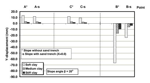
Figure 20. Comparison between additional vertical displacements in slope ( $\beta = 20^{\circ}$ ) for different types of clay soil due to strip load.
