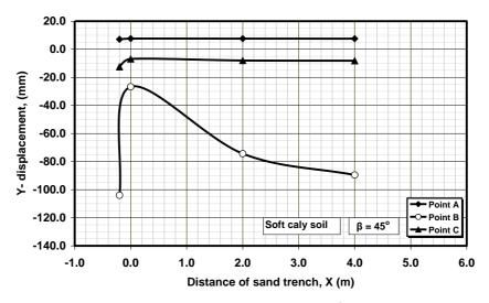
Figure 9. Vertical displacements for slope ( $\beta = 45^{\circ}$ ) due to strip footing, case of soft clay (C = 10 KN/m<sup>2</sup>)
