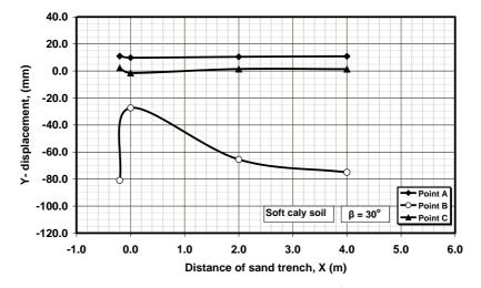
**Figure 10.** Vertical displacements for slope ( $\beta = 30^{\circ}$ ) due to strip footing, case of soft clay (C = 10 KN/m<sup>2</sup>)
