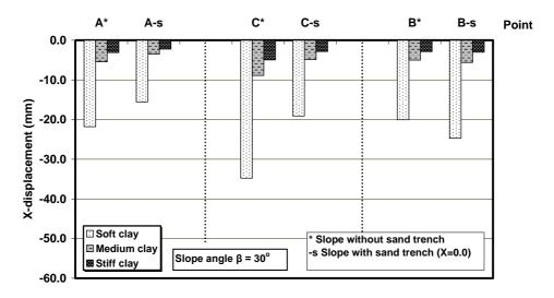
**Figure 14.** Comparison between additional horizontal displacements in slope ( $\beta = 30^{\circ}$ ) for different types of clay soil due to strip load.
