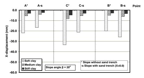
**Figure 15.** Comparison between additional horizontal displacements in slope ( $\beta = 20^{\circ}$ ) for different types of clay soil due to strip load.
