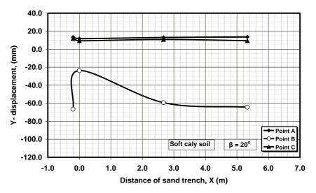
**Figure 11.** Vertical displacements for slope ( $\beta = 20^{\circ}$ ) due to strip footing, case of soft clay (C = 10 KN/m<sup>2</sup>)
