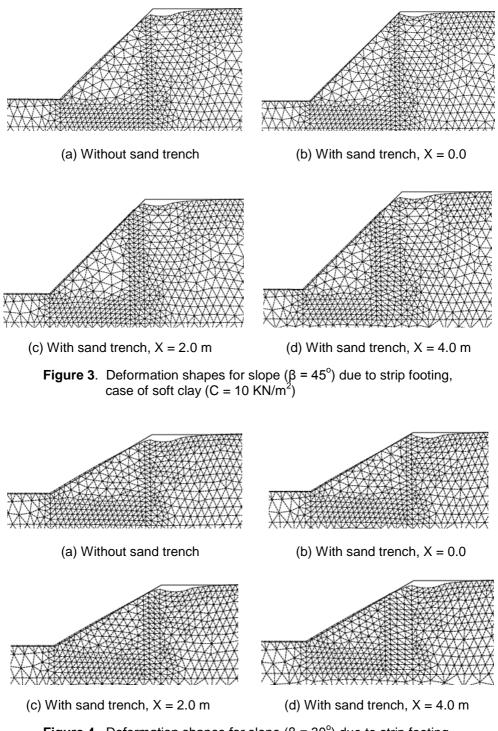
Figure 4. Deformation shapes for slope ( $\beta$  = 30<sup>°</sup>) due to strip footing, case of soft clay (C = 10 KN/m<sup>2</sup>)
