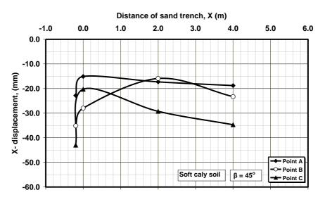
Figure 5. Horizontal displacements for slope ( $\beta = 45^{\circ}$ ) due to strip footing, case of soft clay (C = 10 KN/m<sup>2</sup>)
