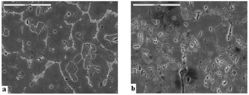
Fig. 6. SEM photomicrographs of the produced Al-Ti-C master alloys at 1000 °C and different reaction times. a) 10 min b) 20 min
