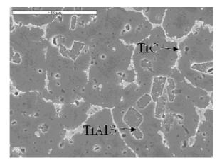
Fig. 2. SEM photomicrograph of the produced Al-4.5Ti-0.6C master alloy at 1000°C
