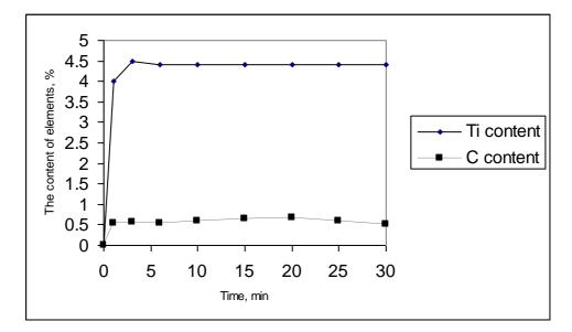
Fig. 8. The relationship between the reaction time and the content of Ti and C in Al-Ti-C master alloys at constant temp. =  $1000 \text{ }^{\circ}\text{C}$ , R= 0.25 and R<sub>1</sub>= 0.01.
