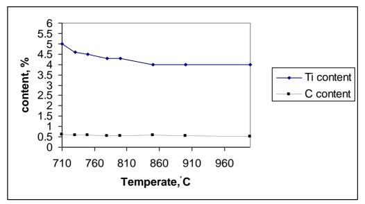
Fig. 9. The relationship between the reaction temperature and the content of Ti and C in the Al-Ti-C master alloys at constant time = 20min, R= 0.225 and R<sub>1</sub>= 0.01.
