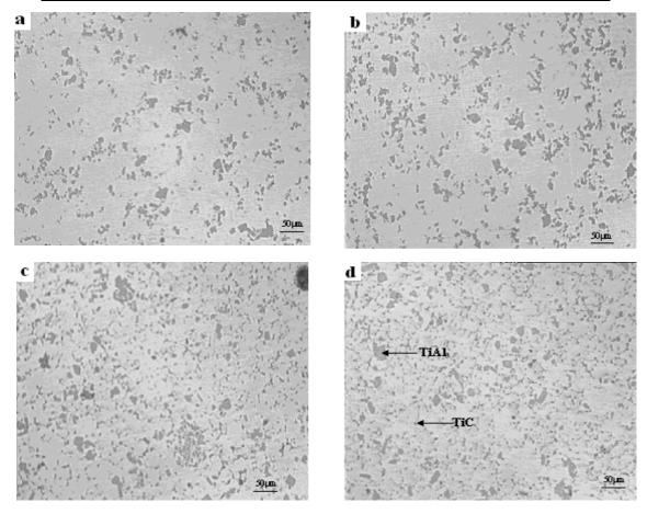
Fig. 5. Optical photomicrographs of the produced Al-Ti-C master alloys at 20 min and various temperatures. a) Al-4.3Ti-0.55C, at 800 °C b) Al-4Ti-0.58C, at 850 °C c) Al-4Ti-0.53C, at 900 °C
