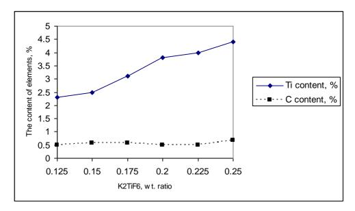
Fig. 7. The relationship between the  $K_2 TiF_6/Al$  weight ratio and the content of Ti and C in Al-Ti-C master alloys at constant temp. = 1000 °C, time = 20 min and  $R_1$ = 0.01.
