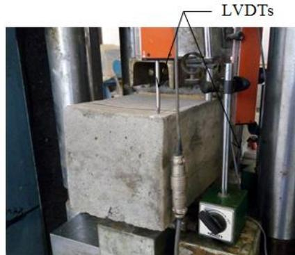
**Fig. 4.** Photo Describing Testing and Instrumentations Setup of Prisms
