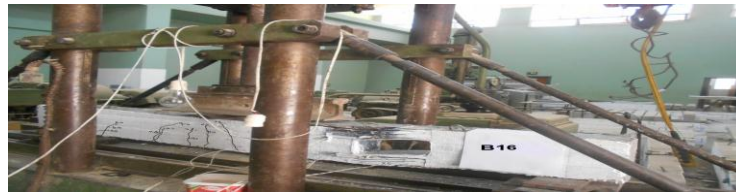
Photo 19. Crack pattern of beam "B16".
