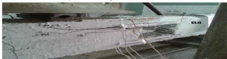
Photo 11. Crack pattern of beam "B8".
