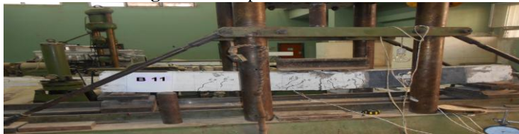
Photo 14. Crack pattern of beam "B11".
