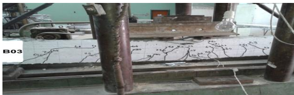
Photo 4. Crack pattern of beam "B03".
