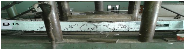
Photo 16. Crack pattern of beam "B13".
