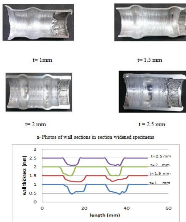
**Fig. 17.** a) Photos and b) thickness distribution plots along section length for different specimens in section widening
