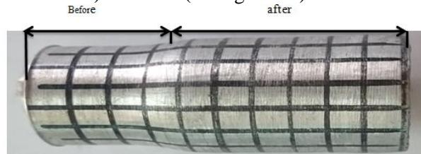
**Fig. 5.** Gridded specimen before and after deformation in tube end widening.
