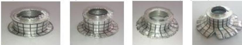
**Fig. 14.** Photos of flanged Al tubes, 2.5 mm thick for varying entry distances
