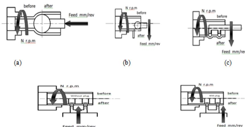
**Fig. 2.** Tube forming processes used in the present work:
