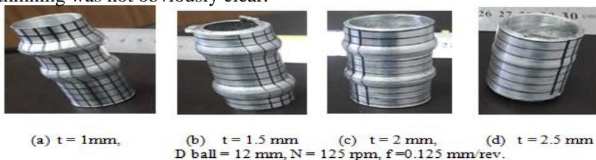
**Fig. 16.** Photos of the in-section widened specimens
