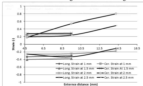
Fig. 24. Variation of the circumferential and longitudinal strains during in-section flanging experiments
