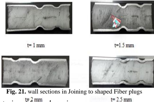
**Fig. 21.** wall sections in Joining to shaped Fiber plugs
