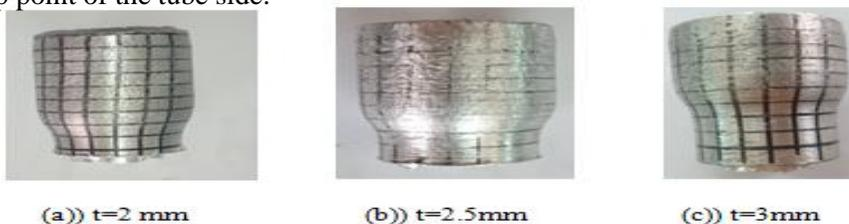
**Fig. 9.** Photos of end-widened tubular specimens using ball diameter of 30 mm
