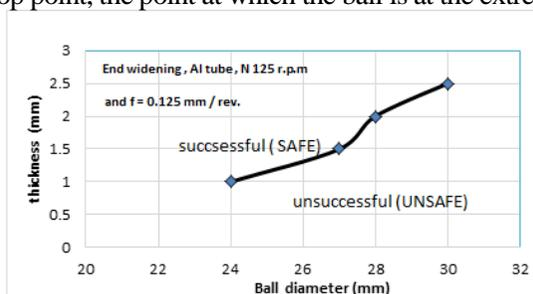
**Fig. 10.** The limit curve in widening of commercial purity Aluminum
