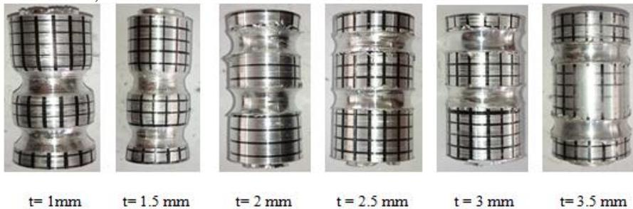
Fig. 18. Photos of the throttled specimens
