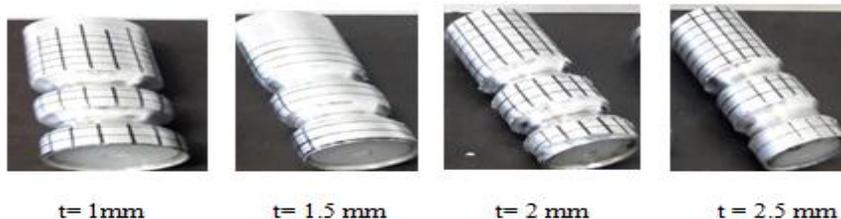
**Fig. 20.** Joining of Aluminum tubes to shaped polymeric (PP) plug
