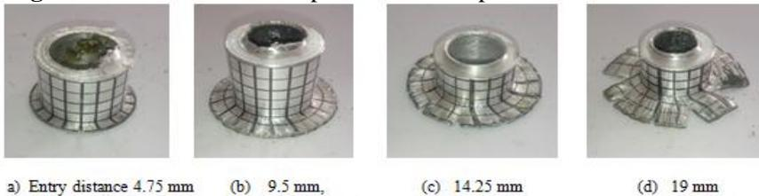
**Fig. 13.** Photos of flanged tubes, 2 mm thickness for varying entry distances
