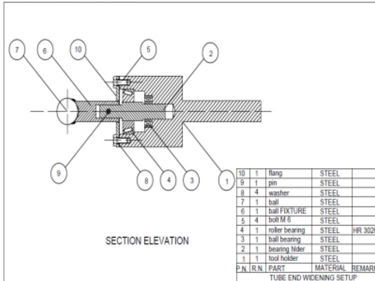
**Fig. 3.** Assembly drawing of the ball-ended forming tool used
