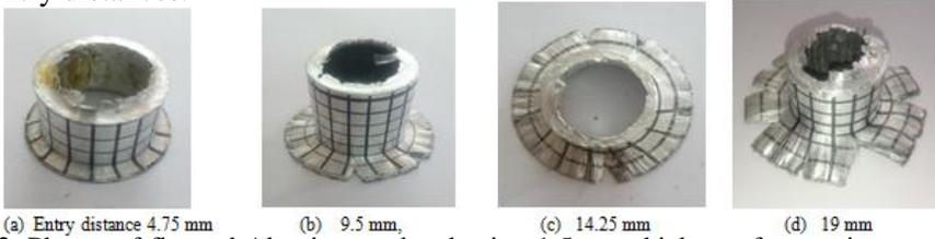
**Fig. 12.** Photos of flanged Aluminum tubes having 1.5 mm thickness for varying entry distance of the 19 mm forming ball
