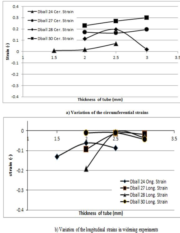
Fig. 22. Relationships between the strain in the longitudinal and circumferential directions for different initial tube thickness values
