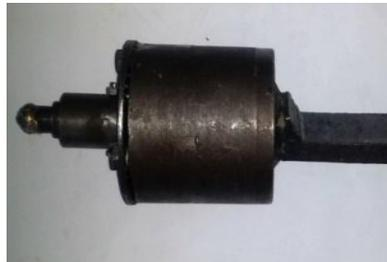
**Fig. 4.** A photo for the assembled ball-shaped Forming Tool
