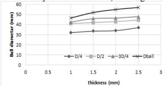
**Fig. 15.** Flange diameter vs. tube thickness in Flanging ( $D_{ball}=19$  mm,  $N=125$  rpm and  $f=0.125$  mm/rev)
