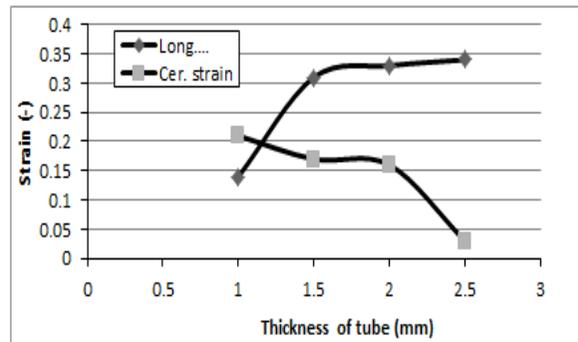
Fig. 23. Variation of the circumferential and longitudinal strains during in-section widening experiments
