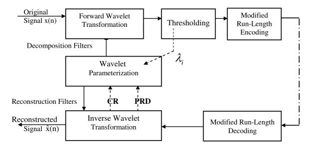
Figure (3) Block diagram for the proposed compression algorithm.
