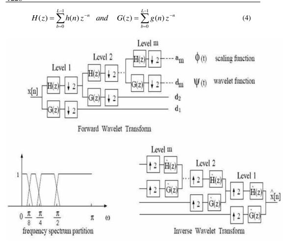
Figure (1) The discrete dyadic wavelet transform as iteration of a 2-channel filter bank.
