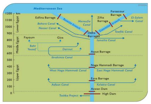
Fig. 2. Schematic diagram of major control structure on the Nile in Egypt [8]
