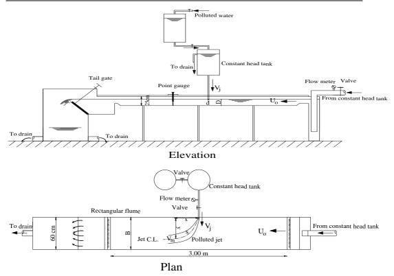
Fig.1: Schematic representation of the experimental set-up.
