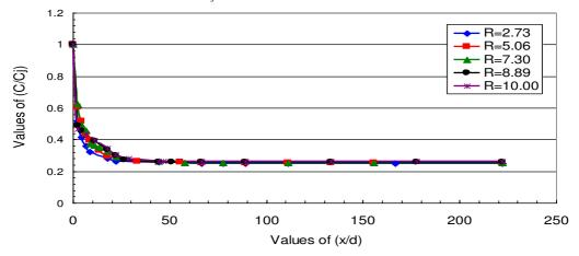
Fig. 7: Relationship between C/C<sub>j</sub> and x/d for different velocity ratios at  $\theta = 45^{\circ}$  and C<sub>j</sub>/C<sub>o</sub> = 4.34.
