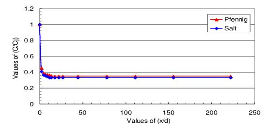
Fig. 6: Relationship between C/C<sub>j</sub> and x/d for different types of pollutants at  $\theta = 90^{\circ}$ , C<sub>j</sub>/C<sub>o</sub> = 2.94 and R = 7.30.
