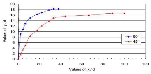
Fig. 3: Influence of jet inclination to the mainstream on jet trajectory for R = 10.00.
