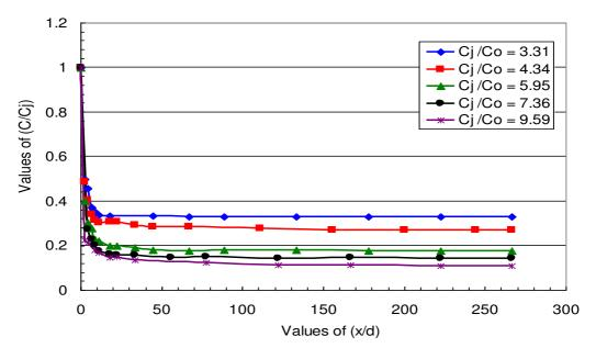
Fig. 8: Relationship between C/C<sub>j</sub> and x/d for different values of  $C_j/C_o$  at  $\theta=90^\circ$  and R=2.73.
