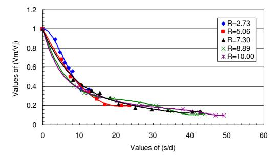
Fig. 5: Decay of centerline velocity-excess for different velocity ratios at  $\theta = 90^{\circ}$ .
