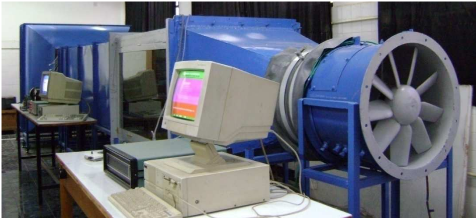
Figure 2: An overall photographic view of the present ABLWT with measuring and control facilities
