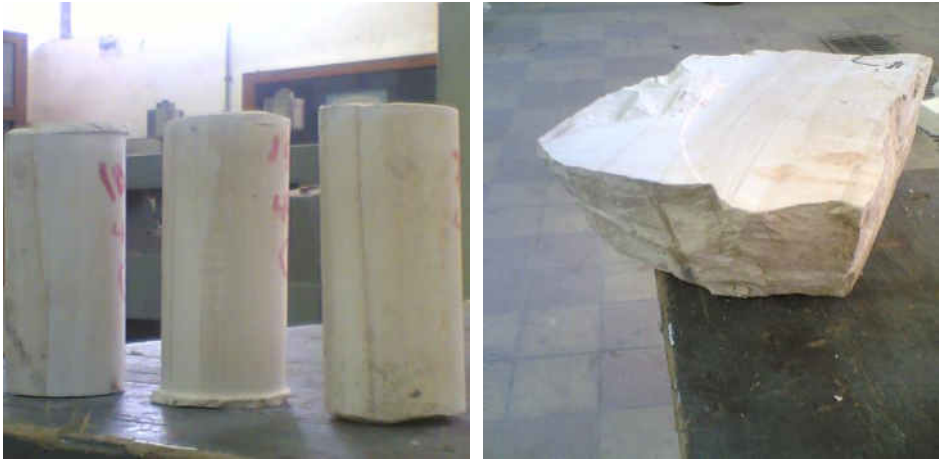
Fig (3): showing core and sample from Bedding limestone
