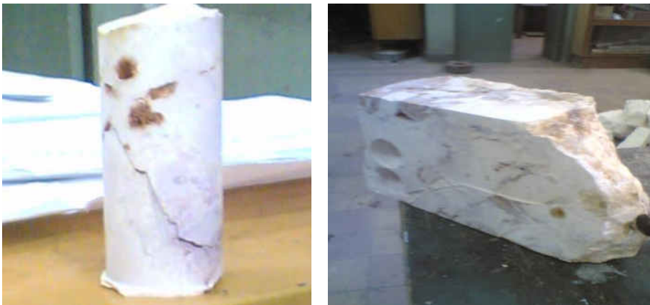
Fig.(5) : showing core and sample from Limestone with interfaces
