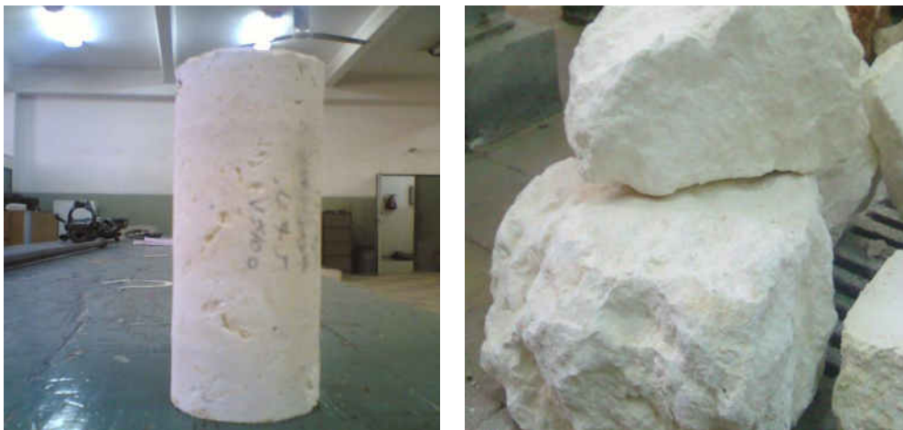
Fig ( 1 ) showing core and sample from fresh limestone
