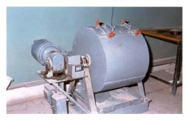
Figure 3: Los Angeles abrasion apparatus
