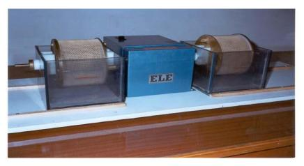
Figure 4 : Slake durability test apparatus
