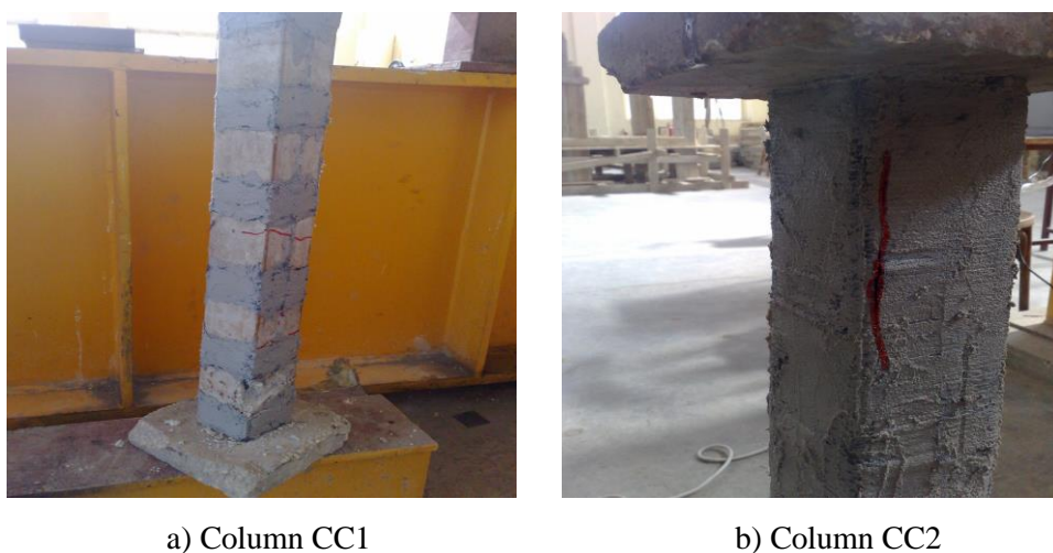
Figure 9: Crack Pattern for Column Strengthened Using CFRP
