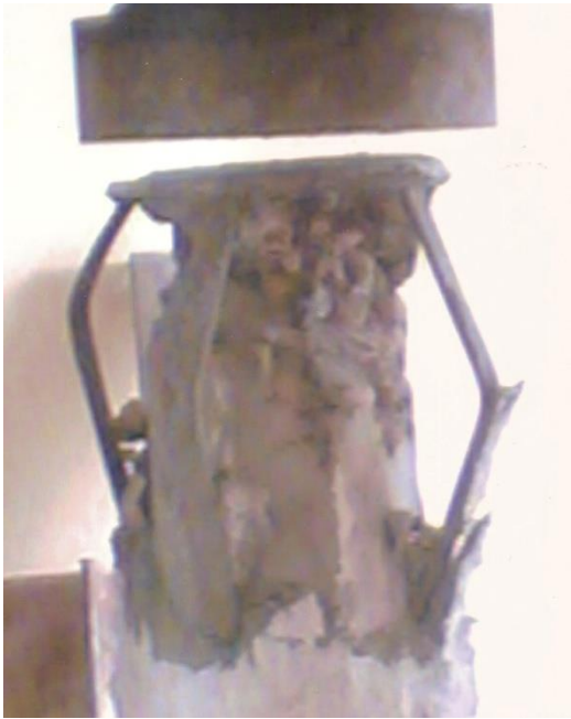
Figure (17) total fracture of the column and the steel jacket of the circular column.
