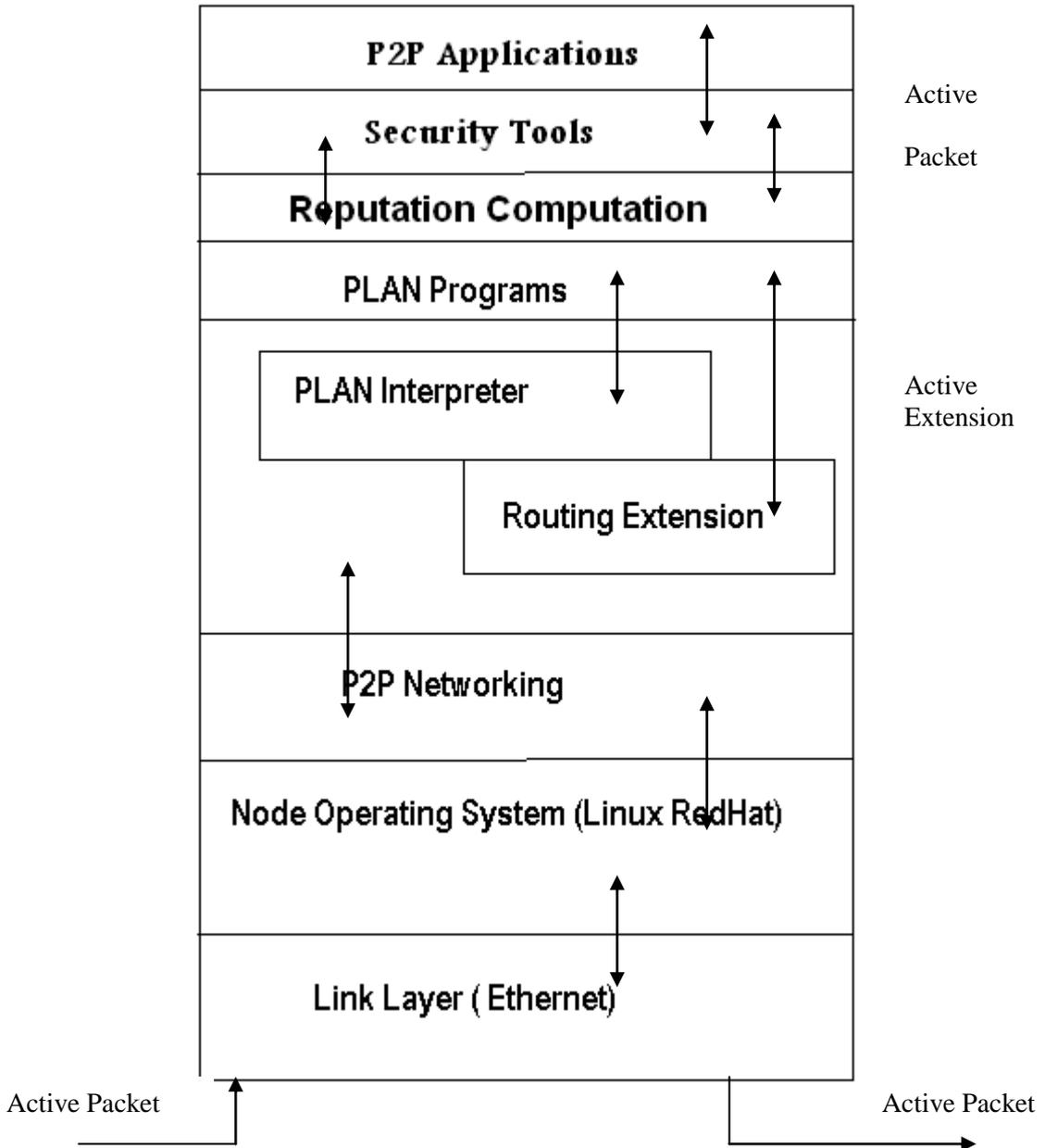
Figure 1: Proposed secure active routing node architecture
