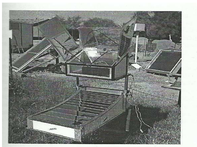
Fig. 2. A photograph of the experimental setup of the double exposure solar cooker of Harmim et al. [8].
