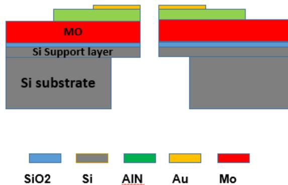
**Fig. 1.** Schematic cross-section of the MEMS AlN Speaker.
