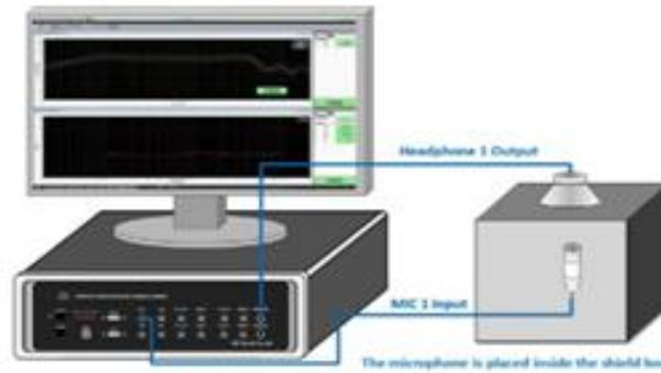
Fig. 6. Photograph for hardware connection of MEMS speaker-test
