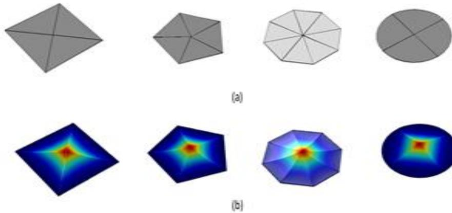
Fig. 2. (A) Different geometries of MEMS speakers with approximately equal size 3 × 3 mm<sup>2</sup>, (b) Simulated displacement of the speakers when applied voltage on the electrodes.
