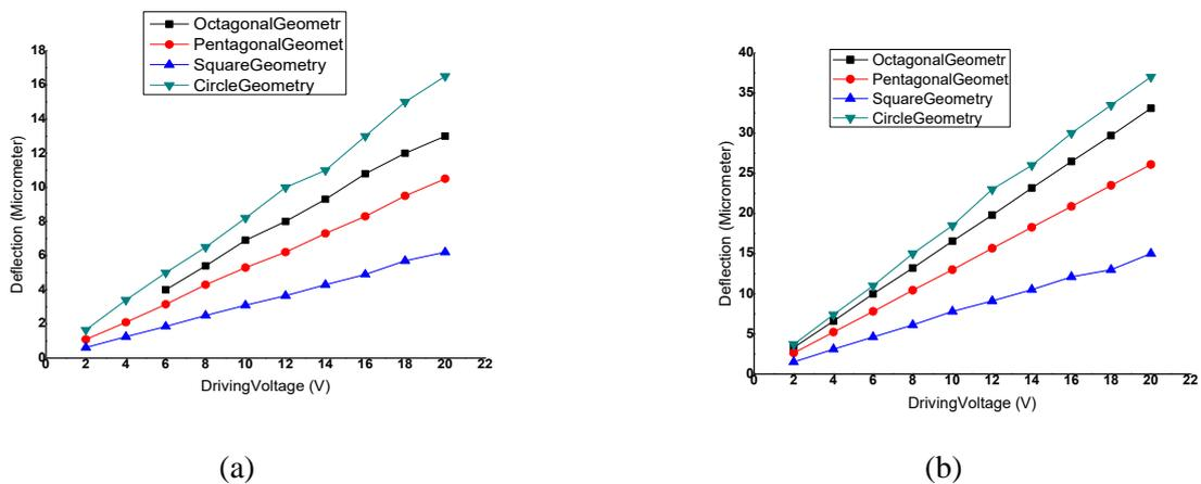
Fig. 3. Maximum deflection amplitude versus driving voltage for different geometries when (a) silicon supporting layer 5 (μm), (b) silicon supporting layer 2 (μm).
