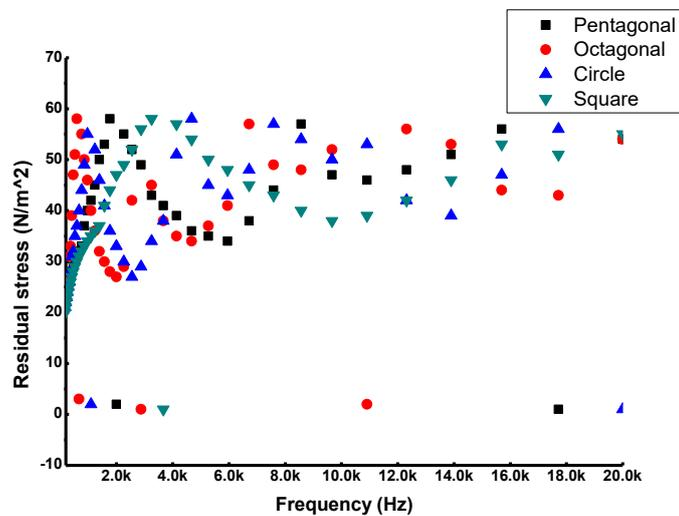
Fig. 4. The simulated residual stress versus audio range frequencies in the different speaker geometries.
