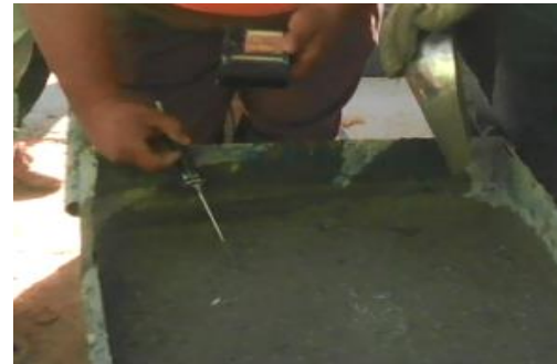
Figure 5: Measuring Concrete Temperature
