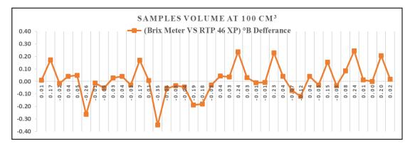
**Fig. 5: Difference of Brix Degree (°Bx) at Samples Volume 100 cm<sup>3</sup>** Max Positive Difference = 0.24 °Bx Max negative Difference = -0.35 °Bx
