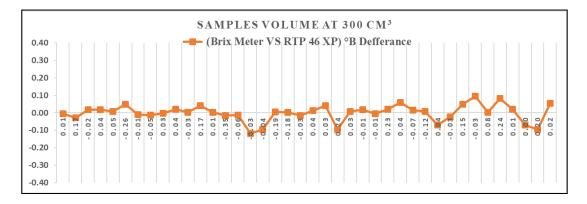
Fig. 7: Difference of Brix Degree (°Bx) at Samples Volume 300 cm³Max Positive Difference = 0.1 °BxMax negative Difference = -0.12 °Bx
