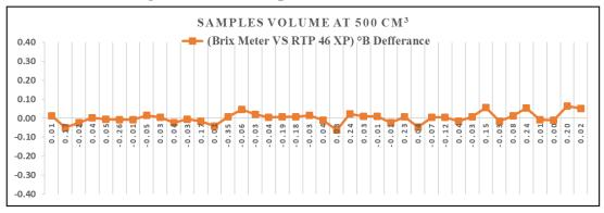
Fig. 9: Difference of Brix Degree (°Bx) at Samples Volume 500 cm³Max Positive Difference = 0.06 °BxMax negative Difference = -0.06 °Bx
