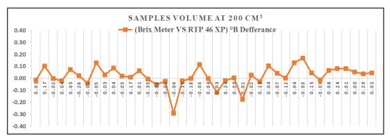
**Fig. 6: Difference of Brix Degree** (°**Bx**) **at Samples Volume 200 cm<sup>3</sup>** Max Positive Difference = 0.17 °Bx Max negative Difference = -0.29 °Bx
