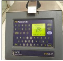
Fig.4: PTR 46 XP Refractometer
