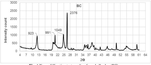
Fig. 1 X-ray diffraction test results of raw ball- clay (BC).
