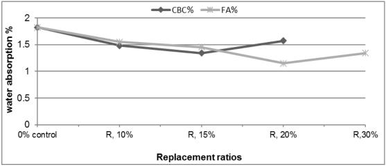
Fig. 9. Concrete water absorption% at different Replacement ratios of CBC and FA.
