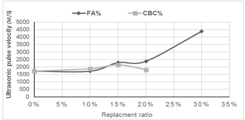
Fig. 11. The effect of FA% and CBC% on concrete ultrasonic pulse velocity at age of 28 days.
