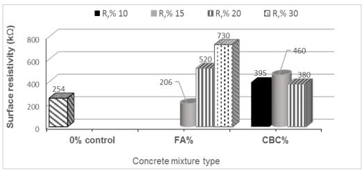
Fig. 10. The effect of FA% and CBC% on concrete Surface electrical resistivity after 28 days of age.
