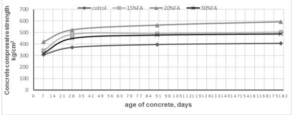
Fig. 7: Effect of fly ash, FA% as partial replacement of OPC on concrete compressive strength.
