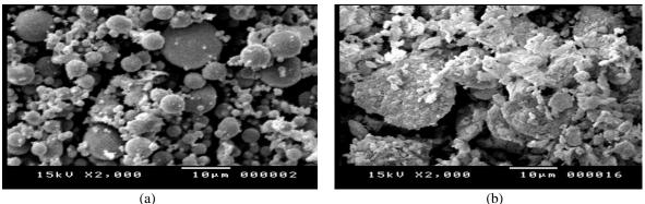
Fig. 2 SEM micrographs of (a) FA and (b) CBC.
