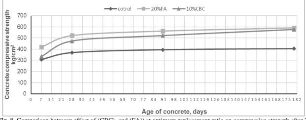
**Fig.** 8. Comparison between effect of (CBC), and (FA)) at optimum replacement ratio on compressive strength after 7, 28, 90 and 180 days.
