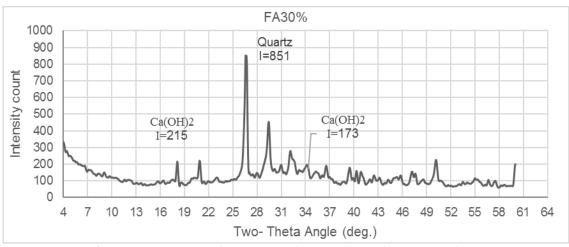
Fig. 14. XRD patterns of OPC paste with 30% of FA after 28 days of age.
