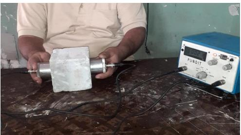
Fig. 4: Experimental Set-up for Ultrasonic Pulse Velocity Testing
