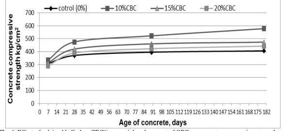
Fig. 6: Effect of calcined ball-clay, CBC% as partial replacement of OPC on concrete compressive strength.
